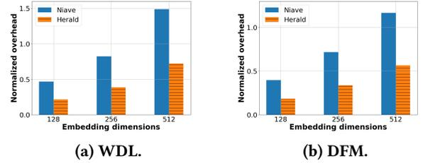
Figure 4: Normalized cache overhead comparison in 25G network.
