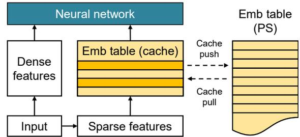
**Figure 1: A typical architecture of cache-enabled embedding models.**
